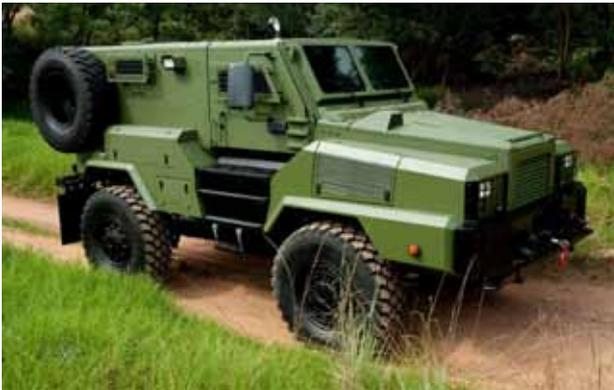
REVA armoured personnel carriers are double-skinned and possess a V-shaped hull, offering occupants superb protection from IEDs.
